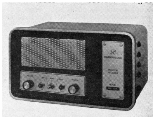
This is an example of the new Hammarlund range of monitor receivers, intended for crystal-controlled fixed-frequency working in the amateur and commercial bands 25-54 mc and 144-174 mc. Selection of up to six channels is provided by panel control, for either NBFM (5 kc deviation) or WBFM (15 kc deviation) depending on model used and service required. The main application of these receivers is in government communications services and on business or industrial radio networks.
