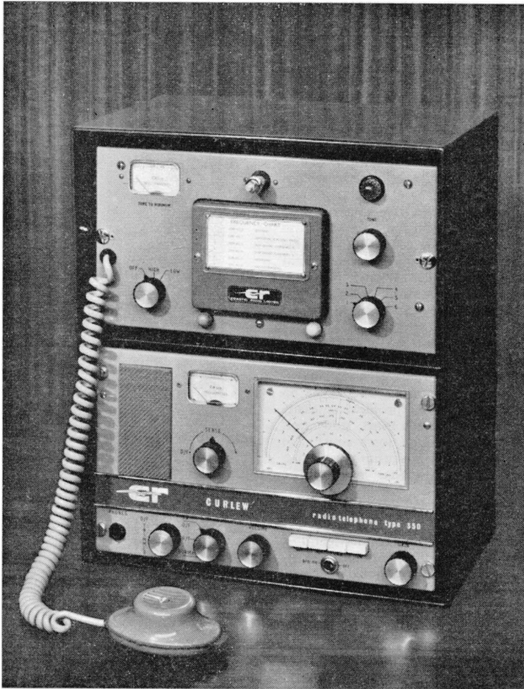
Coastal Radio, Ltd. offer a 65-watt transceiver called the "Curllew," for simplex operation from either a 12v. or 24v. DC supply. The receiver tunes 170-425 kc, 600-1600 kc, and 1.6-4.0 mc, with an optional D/F facility; the S-meter as fitted functions also as a null-indicator when using the Consol position-finding system. A BFO for CW reception and a headphone jack are provided. The Tx coverage is 1.6-4.0 mc in six CC channels, the valve line being N78-QV06-20 in the CO-PA, and N78-2/QV06-20 in the speech amp.-modulator, using a good-quality carbon microphone. The PSU is a DC/DC converter with 2/CT308 power switching transistors. The total load on a 12v. DC supply is about 12 amps.
